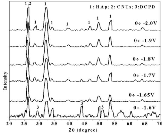
Figure 4. XRD patterns of HAp/CNTs synthesized with the variation of the potential ranges.
