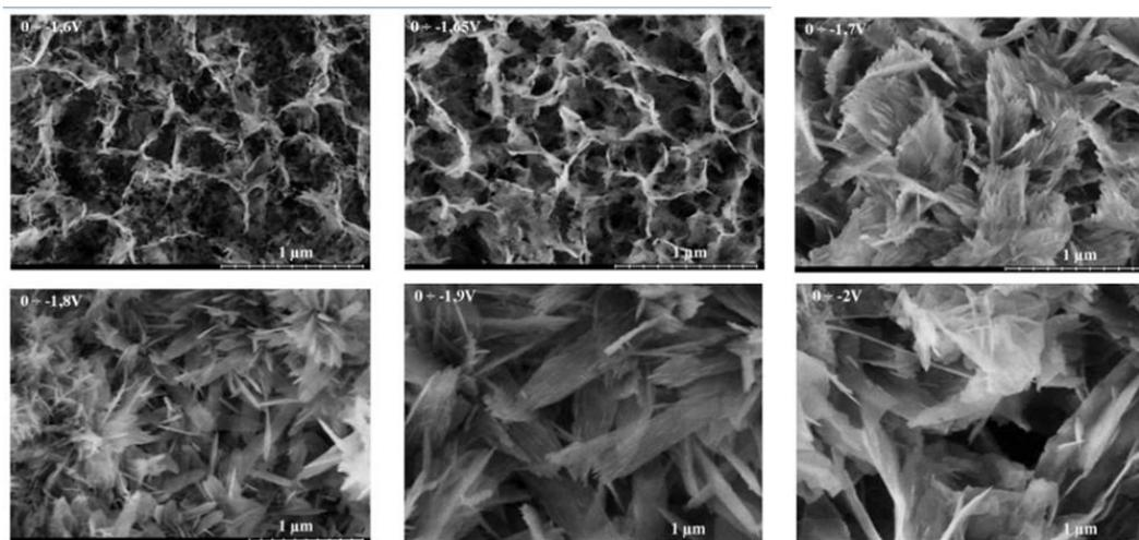
Figure 3. SEM images of HAp/CNTs synthesized with different potential ranges at  $45\text{ }^\circ\text{C}$ .
