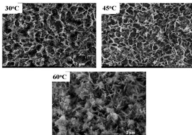
Figure 7. SEM images of HAp/CNTs/316L SS synthesized at different temperatures.
