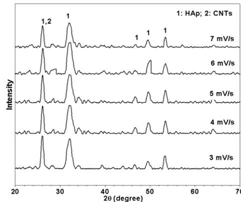
Figure 9. XRD patterns of HAp/CNTs synthesized with different scanning rates.
