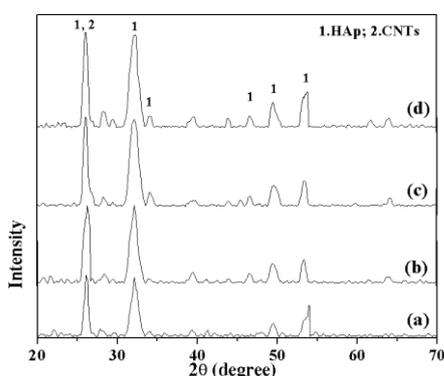
Figure 8. XRD patterns of HAp/CNTs synthesized with different scan numbers: (a) 3; (b) 4; (c) 5 and (d) 6 scans.
