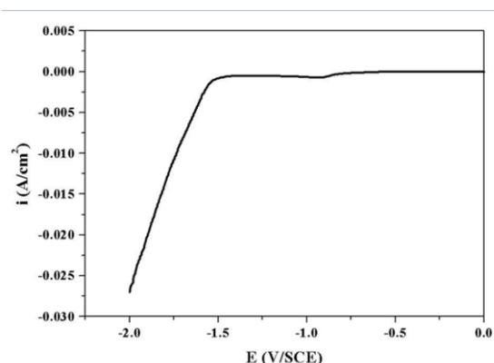
Figure 1. Cathodic polarization curve of 316L SS in the synthesis solution.
