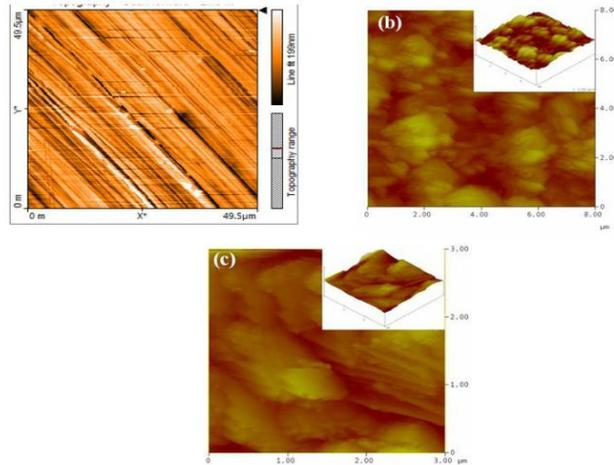
Figure 10. AFM images of (a) 316L SS, (b) HAp/316L SS and (c) HAp/CNTs/316LSS.
