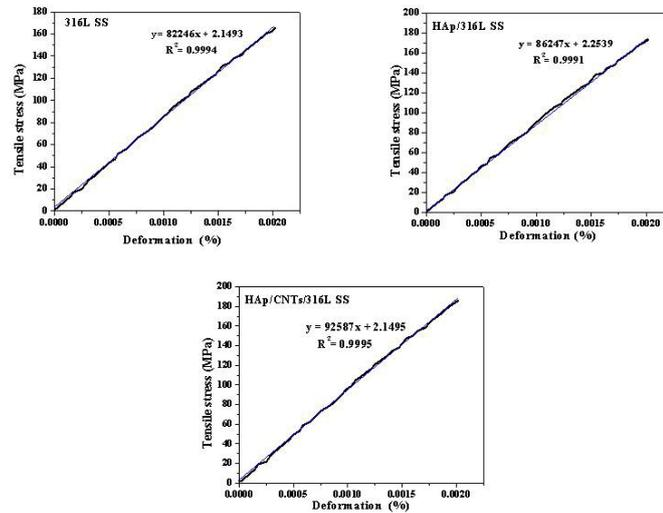
Figure 11. Relationship between the tensile stress and the deformation of the materials.
