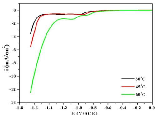
Figure 5. Cathodic polarization curves of 316L SS in the synthesis solution at different temperatures.
