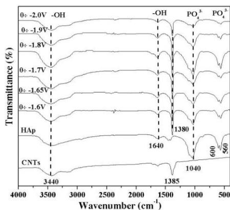
Figure 2. FTIR spectra of HAp/CNTs obtained with different potential ranges at  $45\text{ }^\circ\text{C}$ .
