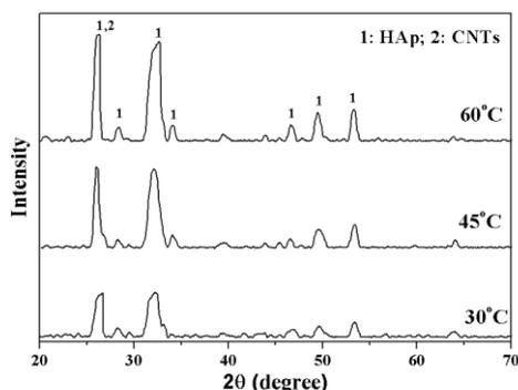
Figure 6. XRD patterns of HAp/CNTs in function of the temperature.
