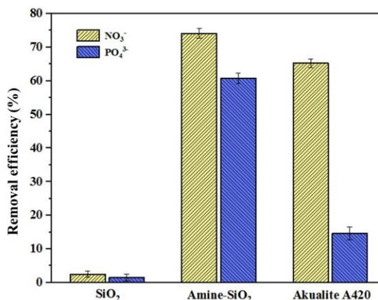
Figure 4. Nitrate and phosphate removal efficiency of adsorbent materials (n = 4).
