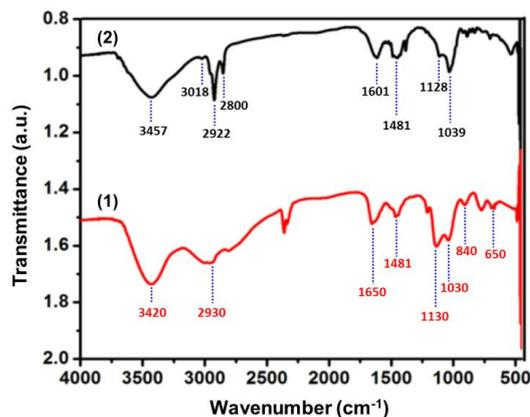
Figure 2. FTIR results of (1) Amine-SiO<sub>2</sub> and (2) Akualite A420.
