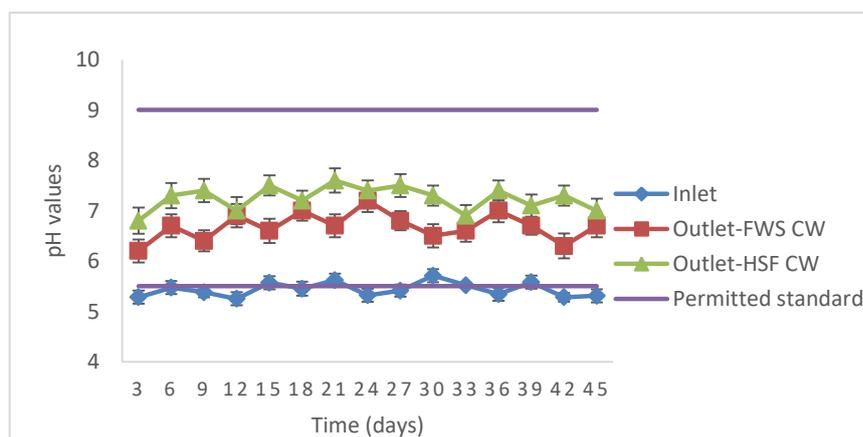
Figure 2. pH values in inlet and outlet of CWs.
