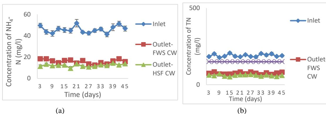
Figure 5. NH<sub>4</sub>-N (a) and TN (b) concentrations in the wastewater inlet and outlet of CWs.
