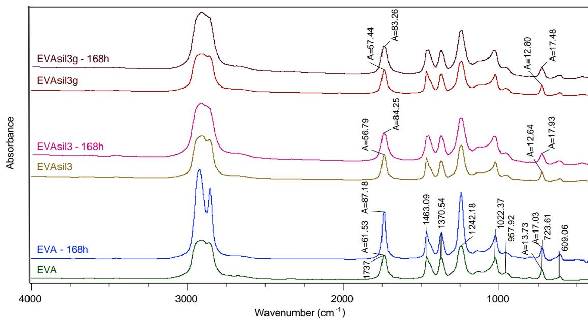
Figure 2. FTIR spectra of EVA and EVAsil3, EVAsil3g before and after thermal oxidative aging.
