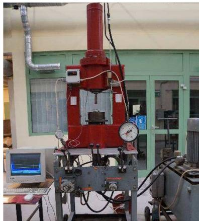
Figure 3. Hydraulic piston press.
