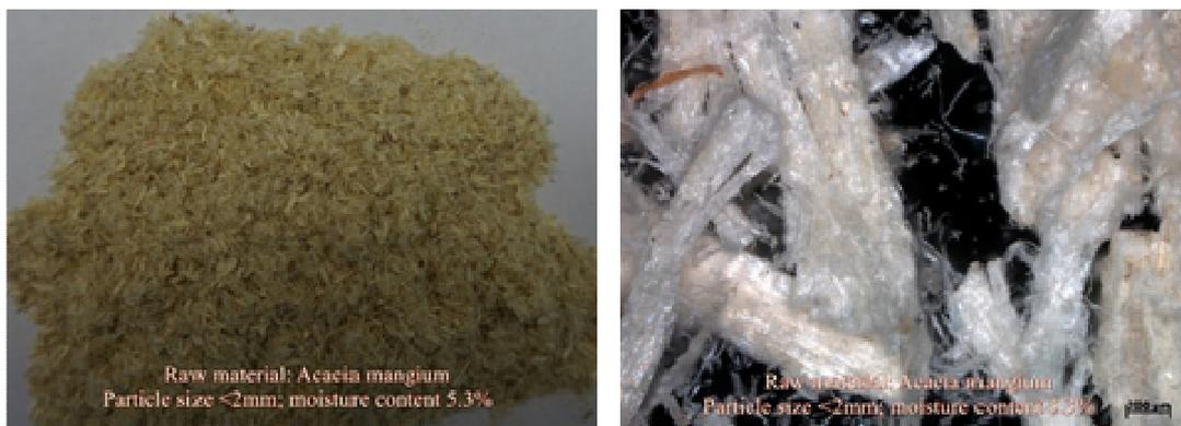
Figure 2. *A.mangium* sawdust with particle size < 2 mm; (left) optical camera; (right) optical microscope: Zeiss AXIO Imager.M2m.
