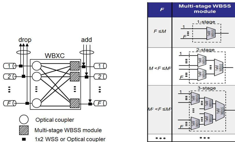
Figure 1. Proposed 1xM WBSS-based waveband cross-connect architecture
